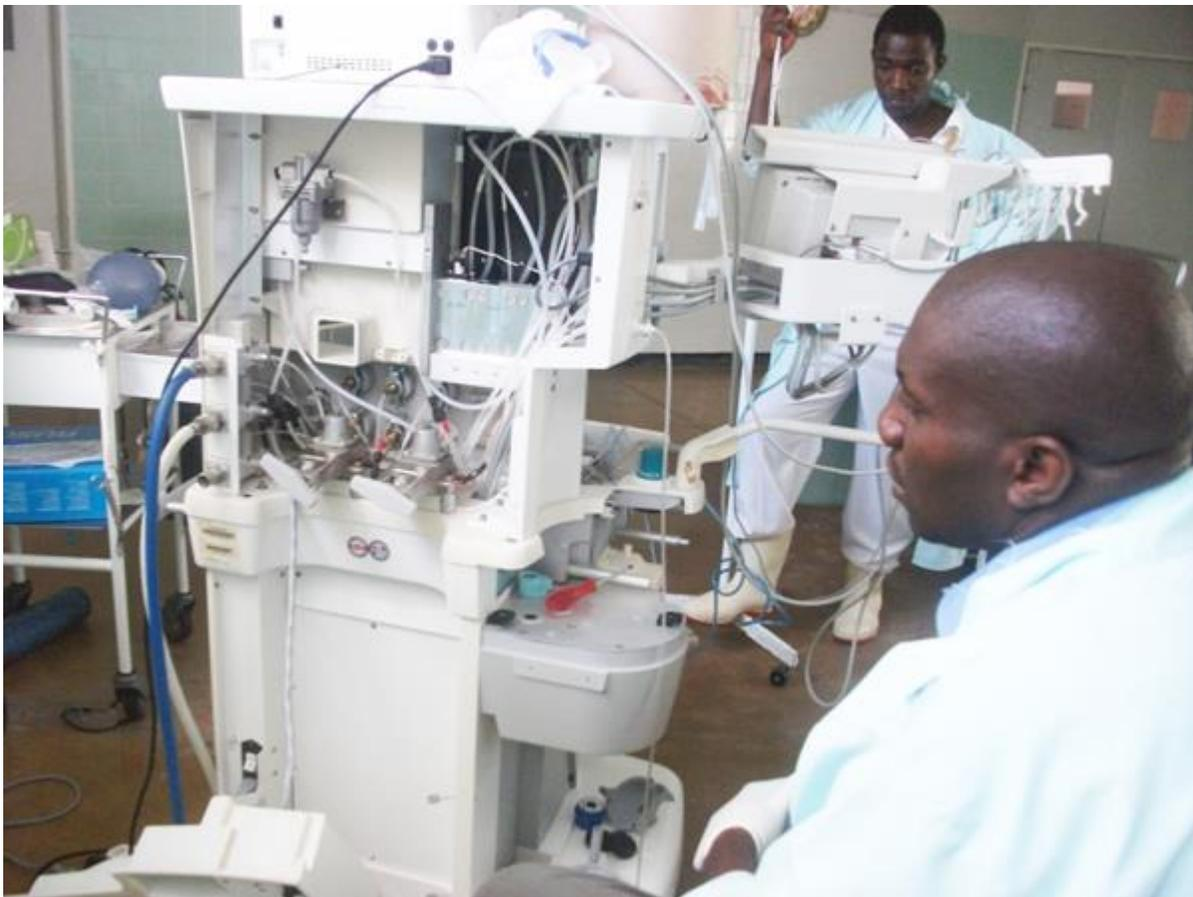
Anesthetic machine under repair
